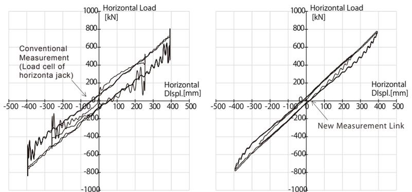
Figure 6. Force – displacement hysteresis loops of seismic isolator (vertical load 16929kN, 2.5Hz sine loading).
