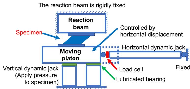
Figure 1. Typical components and conventional force measurement system in dynamic testing machine.
