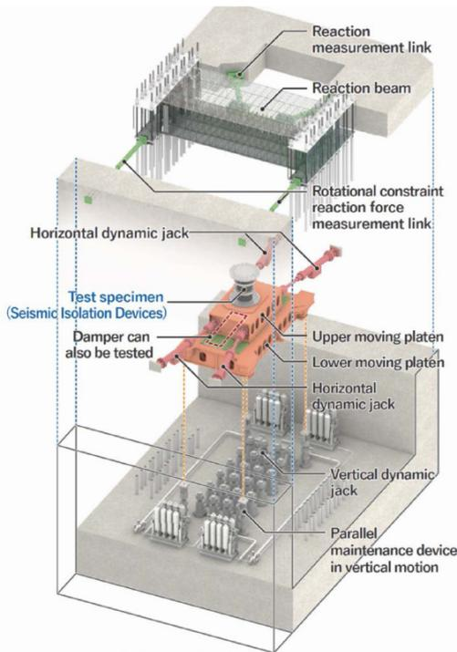
Figure 4. Configuration of E-Isolation.
