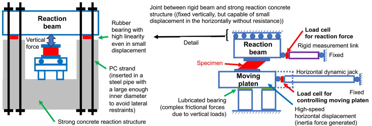
Figure 3. Reaction force measurement system (measurement link and reaction beam support).
