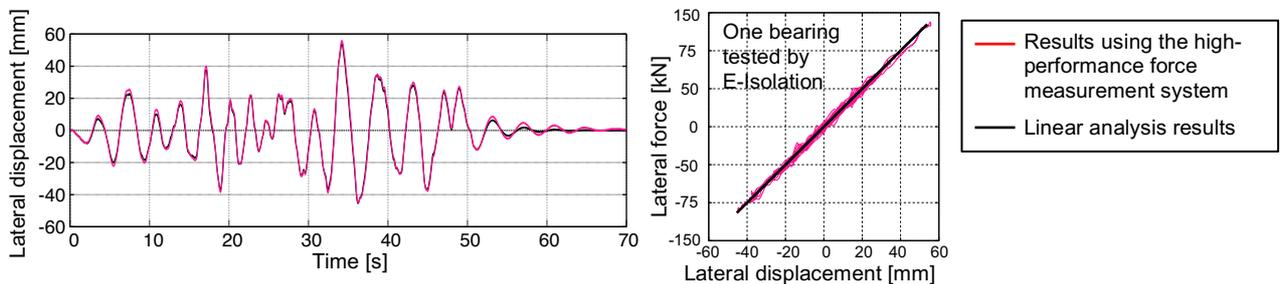
Figure 9. Results of the real-time hybrid simulation using 1200mm-diameter seismic isolator.
