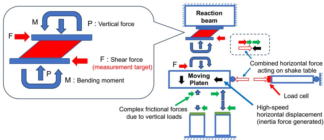
Figure 2. Force acting on moving platen by horizontally deformed seismic isolation bearing.
