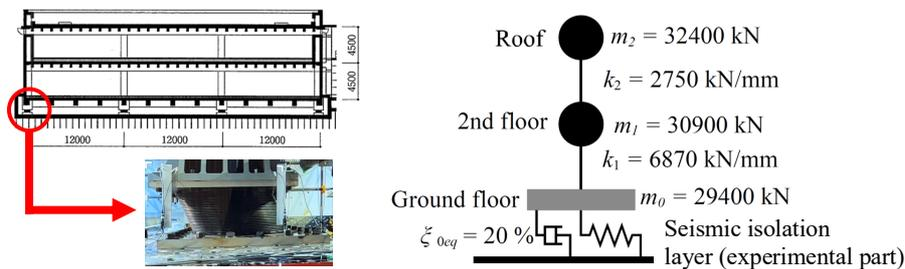
Figure 7. The objective 2-story building and numerical model.
