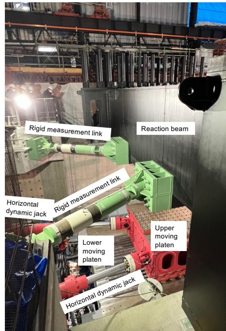
Figure 5. High-performance force measurement system in E-Isolation.
