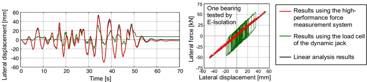
Figure 8. Results of the pseudo-dynamic simulation using 800mm-diameter seismic isolator.
